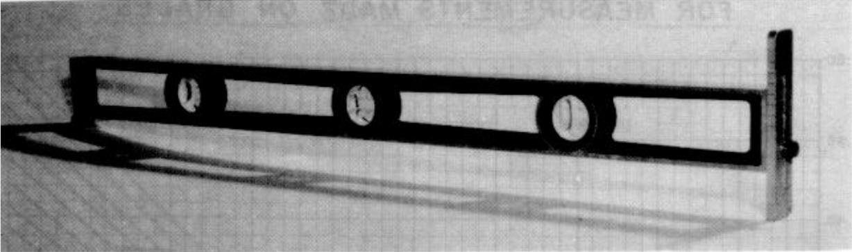
FIGURE 4 - LEVEL FOR MEASURING PAVEMENT SLOPE
